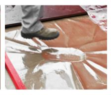
after 24 hours the load-bearing capacity of Egcovoid® is eliminated
