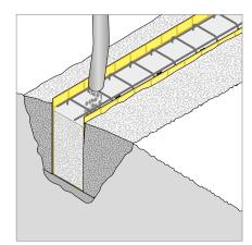
Permanent formwork is sacrificial and the finished concrete surface is usually hidden, which sometimes means **latent** defects e.g. loss of cover, honey-combing and voids may go undetected.
