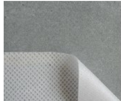
Concrete surface after application from MAX FRANK formwork liner self-adhesive.
