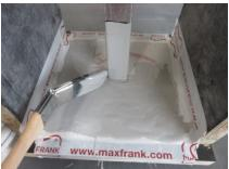
c) After curing of the liquid plastic (24 hours), the formwork of the test specimen is closed and filled with a concrete (grade C30/37(.
