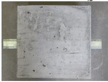
d) After 5 days, the specimen shall be stripped and a test bell shall be applied.
