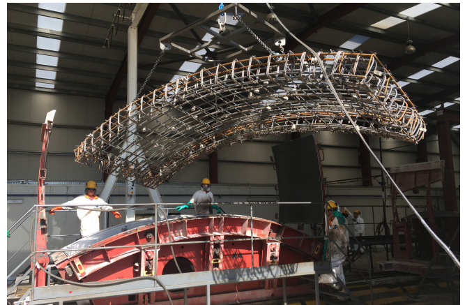
Introduction of reinforcement with fixed spacers into the vibrating formwork © www.maxfrank.com
